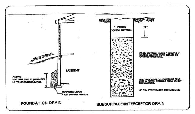
It is a good practice to install subsurface drains, which are at least 4 inches in diameter and are surrounded with gravel or sand. If at all possible, the drain pipe should have 2 feet of cover.
